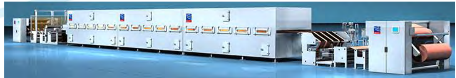
B&W Gigacoater – Roll to Roll 3 Ghr/yr simultaneous double sided coater-dryer
