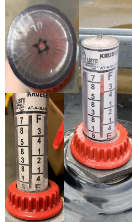
Plastic is cracked in multiple places.
