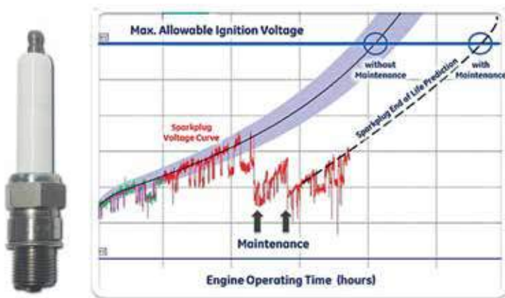
Example of how the remaining useful lifetime of spark plugs is predicted
