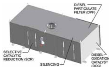
Figure 7: Example of a Multi-Function Exhaust System in a Single cube
