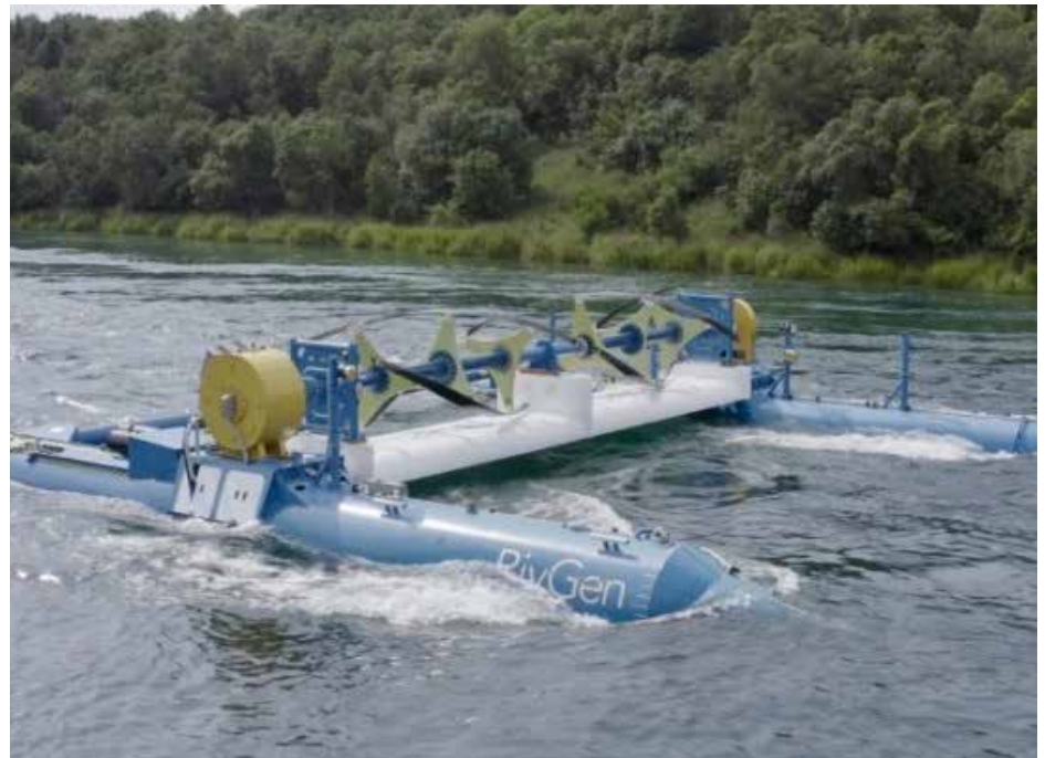
ORPC RivGen Power System before submersion deployment. The device is 15.7 meters long, 14.3 meters wide, and 3.5 meters tall. Credit: ORPC
