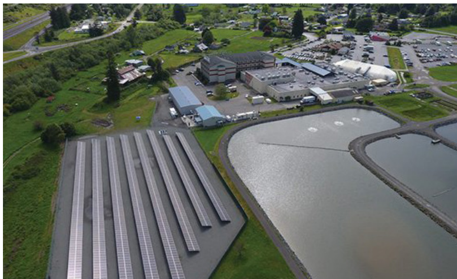
1. The Blue Lake Rancheria microgrid can operate islanded from the main utility grid. A solar array, battery storage, and a Siemens microgrid controller—the Spectrum Power Microgrid Management System—are integrated in the system. Courtesy: Siemens
